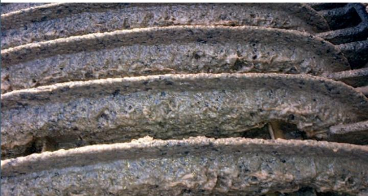
This image shows the large quantity of biomass attached to the 50mm thick mesh plates. Bacteria culture analyses and enzyme studies demonstrate that the biomass is much more active than conventional mixed liquor.
