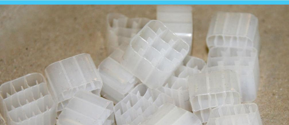
The CFIC reactor contains highly packed biofilm carriers (typically 90-99% bulk volumetric fill) that hinders movement of the carriers that normally occurs in an MBBR reactor.
